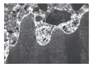
Figure 6 – OM image of cross-section of GFRP from Chatham Bridge.
